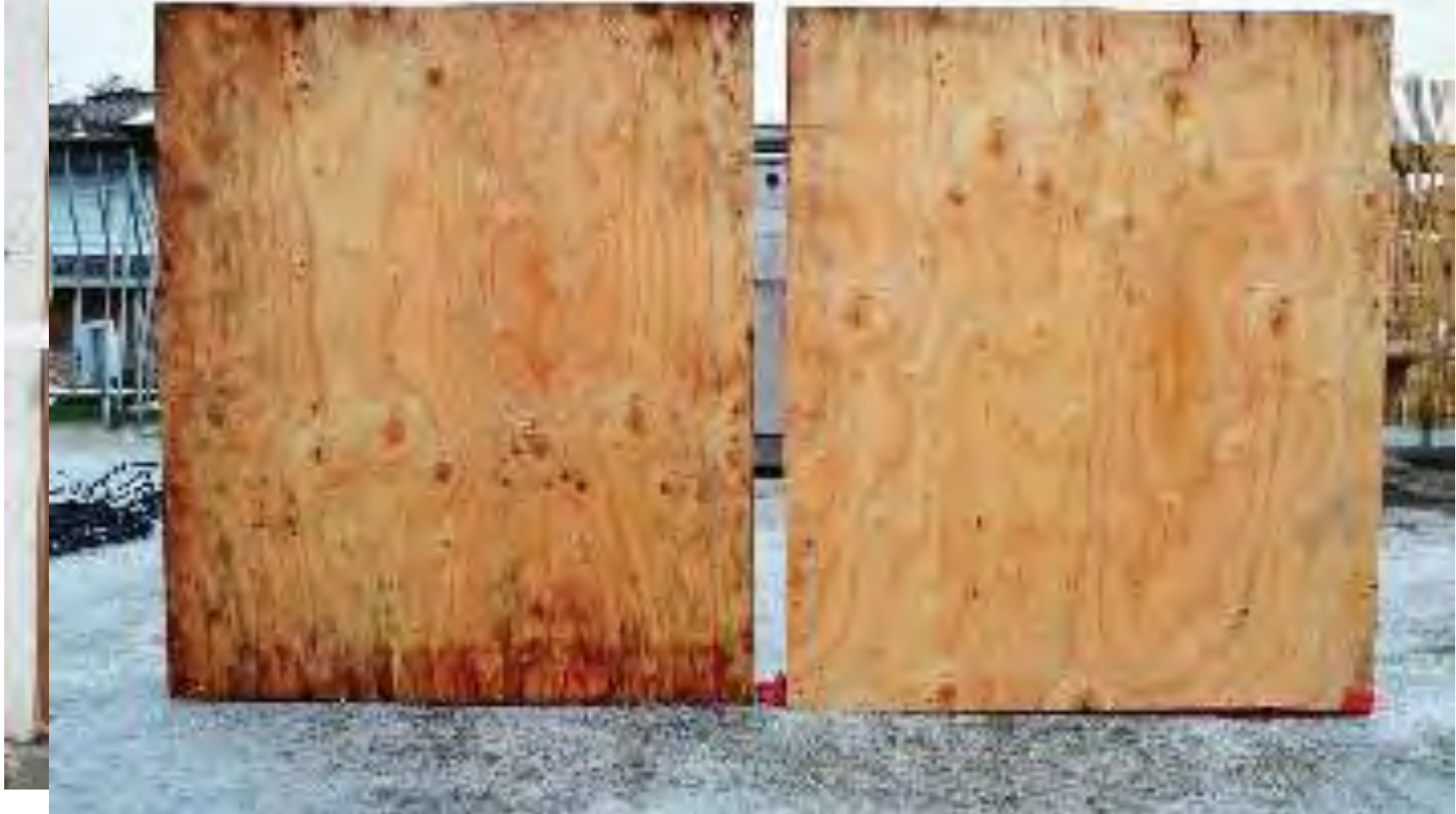
Plywood Behind XPS – wet for 8 weeks
