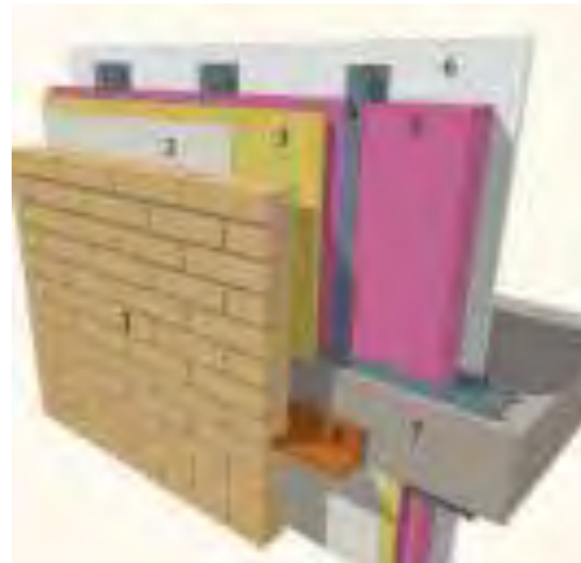
Steel stud wall assembly with concrete slab R 3 – 4 effective
