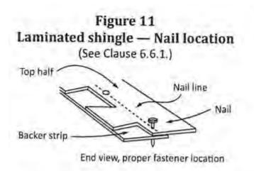
The reasoning behind the RGC requirement is simple: shingles stay put when they are nailed through the laminated region. Nails installed above the common bond risk shingle detachment and product failure.
