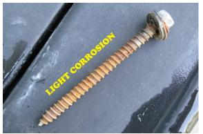
That standard test method is the ASTM B117 Salt Spray Method, and the result is determination of a time period before corrosion can occur. A coating is designed for "X" amount of exposure with a 5% salt spray environment. According to published Grabber Construction Products, they found on average the US standard is a 24-hour requirement, Germany is 48-hours, and Scandinavia is a 96-hour requirement.
